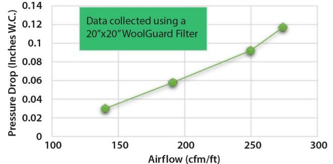
WoolGuard NaturalSorb Panel Filter pressure drop through wool filter only as a function of exhaust. The pressure drop across the WoolGuard shall be 0.1" or less of H<sub>2</sub>O with face velocity of 250 feet-per-minute.
